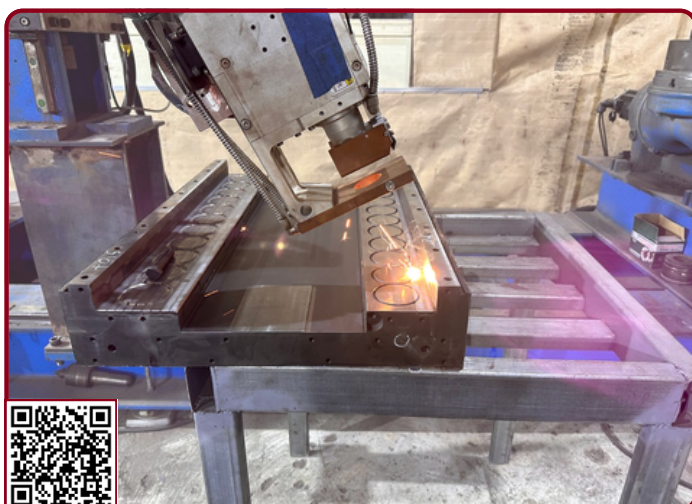
Moving guideway of the boring machine bed
