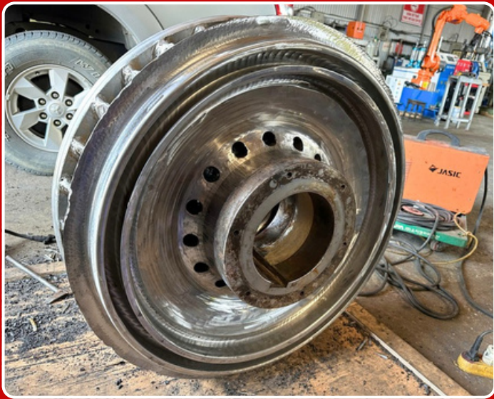
Turbine Runner – Nam Ho Hydropower Restoration: Cracks on the Blades and Runner Body
