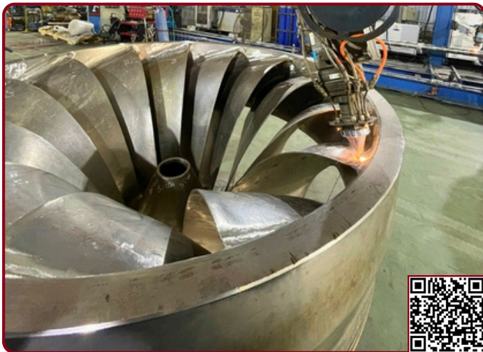
Turbine Runner – Nam Ho Hydropower Restoration: Cracks on the Blades and Runner Body
