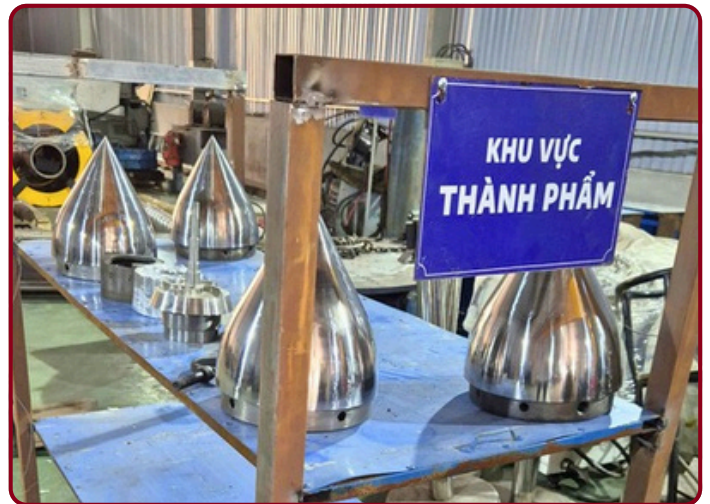
Injection Nozzle – Huong Son Hydropower
