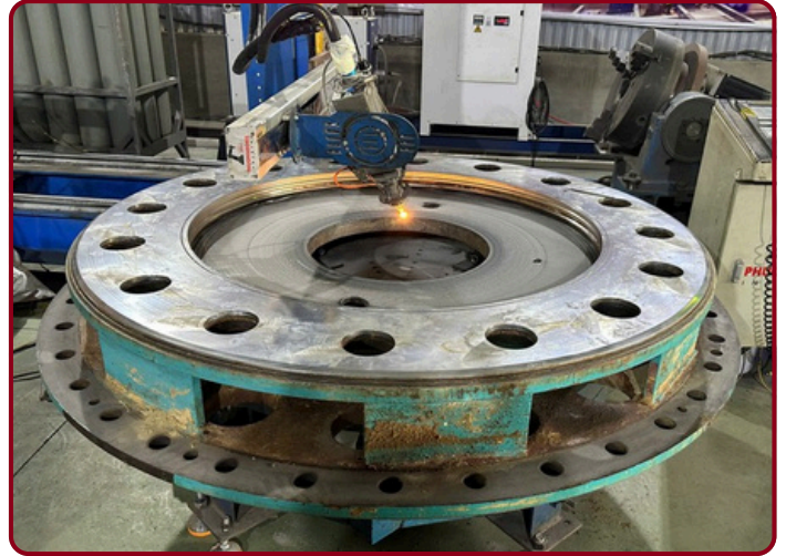
Turbine Cover Seal Ring – Ho Bon Hydropower
