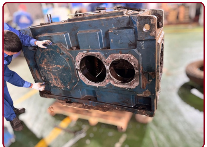
Pellet mill gearbox
