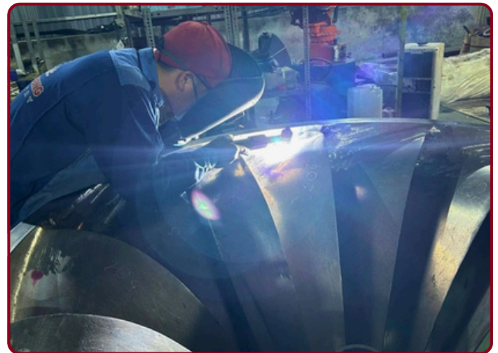
Turbine Runner – Nam Ho Hydropower Restoration: Cracks on the Blades and Runner Body
