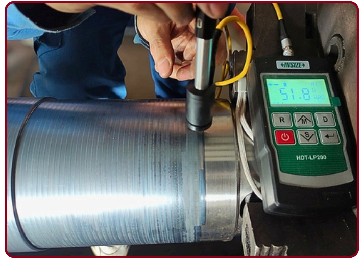
Hardness testing after Laser Hardening
